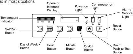
Manual mode - push *On/Off* button - refrigeration compressor will start and run, green Compressor-on light will illuminate. In this mode compressor will run continuously and will not be turned on and off by the monitor. MANUAL OVERRIDE will appear on interface panel.
