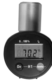
READING BEFORE FILTERING (70.2% Relative humidity)
