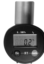
READING AFTER FILTERING (.2% Relative humidity)
